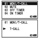
To access a repeater, press and hold in the  $\widehat{\text{}_{\text{T-CALL}}^{\text{MONI}}}$  key for the amount
