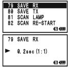
5. When you have made your selection, press the **PTT** switch to save the new setting and exit to normal operation.
