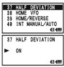
The "normal" setting for the deviation (when this Set Mode Item is set to "OFF") is  $\pm 5 \text{ kHz}$ .
