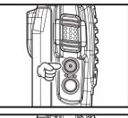
□ To transmit, monitor the channel and make sure it is clear.
