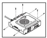
**5** Carefully lift up the front side of the main body top cover
