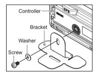
3 Peel off the protective seal from one side of the provided two-sided adhesive sheet, and paste it onto the bottom of the bracket
