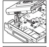
**7** Refer to the figure on the right to mount the FVS-2 Caution Check the direction of the connector and plug the FVS-2 in all the way to the back.
