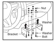
4 Fasten the main body to the bracket, using the provided flange bolts, as shown in the drawing
