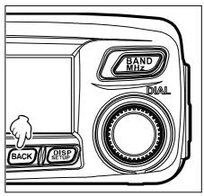
**2** Rotate the DIAL to select the station you want to delete, then press (SETUP).
