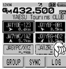
4 Rotate the DIAL, then touch [PICT]. Displays the list of image data saved on the microSD memory card.
