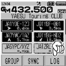
4 Rotate the DIAL, then [MESSAGE] or [PICT]. Select the data type (MESSSAGE or PICT) you want to send. Displays the LOG list.
