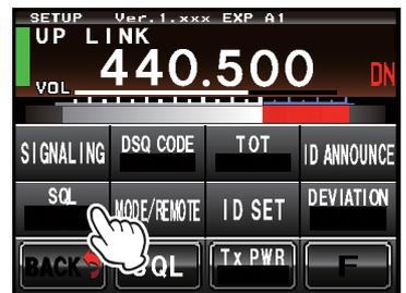
3 Select [RX SQL] to set the tone signal type during reception, or select [TX SQL] to set the tone signal type during transmission
